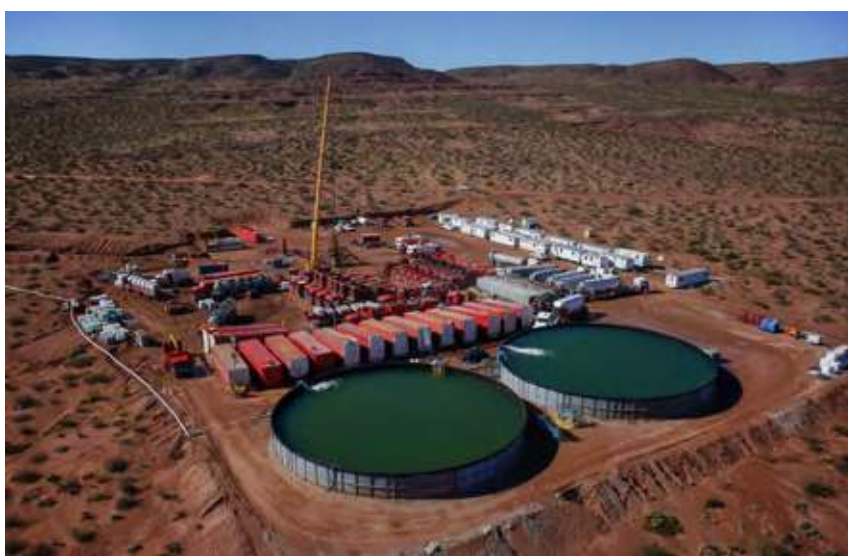
A battery of pumping trucks for fracking at Vaca Muerta shale field in Argentina, August 2014. Photo by SobrevolandPatagonia/Adobe Stock 366388349. Received from FARN, October 2024.
